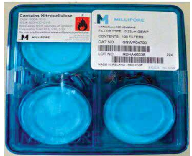
Figure 3. Millipore filter paper with pore size 0.22 micrometre
